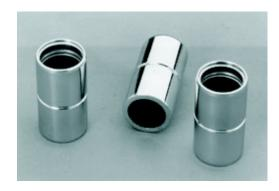
The use of tubes (instead of bars) for these applications not only reduces machining requirements but also increases the fatigue life of the final product because of the better grain structure of tubes. Moreover, tubes are lighter and easier to handle than bars and therefore reduce handling time and associated transportation costs.
